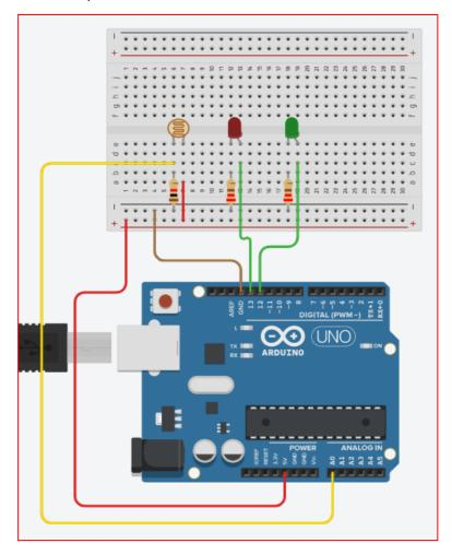
Don't forget the yellow and red wires that are on the left hand side of the Arduino – the red wire provides power to the photoresistor, and the yellow wire lets the Arduino read in how dark it is – the value of the photoresistor.
