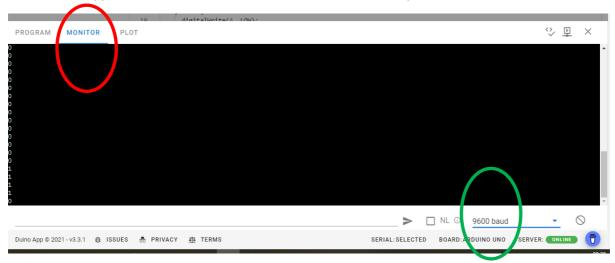
Make sure it is set to 9600 baud rate (circled in green) – this sets the speed for serial communication with the Arduino.
