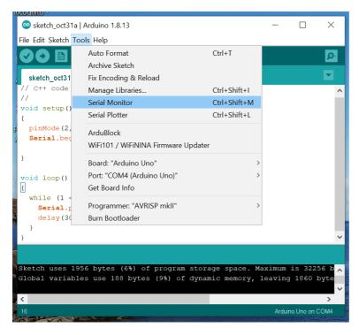
This opens up a new window, with the serial monitor – you can clear the serial monitor using the "Clear output" button.
