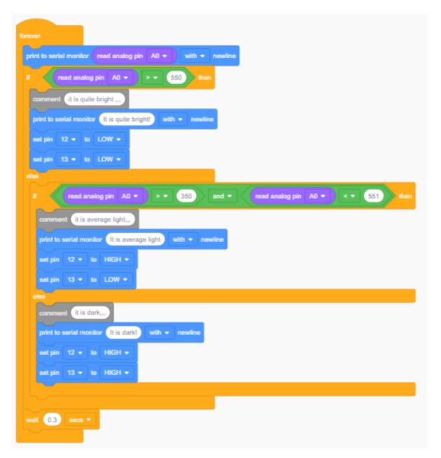
The block "print to serial monitor" means we can tell what value the photoresistor is telling the Arduino, as it will print that value to the screen – there are some more details about this at the bottom of this worksheet. You'll also notice we've put in some comments. Comments are really useful in your code – the Arduino ignores them, but they tell us (and other people!) what you are trying to do in your code.
