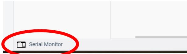
If you’re using a physical Arduino and the IDE, you can see the Serial Monitor by clicking on the **“Tools”** menu and choosing **“Serial Monitor”**. In the Duino App, you can see the Serial Monitor by clicking on the **“Monitor”** tab.
