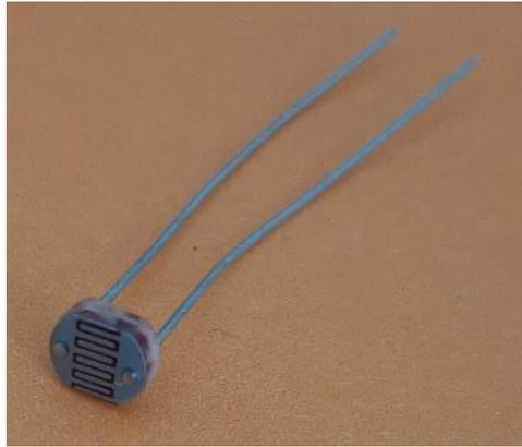
To start with, let's build a circuit that makes our LEDs turn on when it gets dark. There are two circuits: one output circuit (with the LED), and one input circuit (with the photoresistor). As you can see, the photoresistor needs another resistor to work properly – use a 1 k $\Omega$  resistor for this. Use 220  $\Omega$  resistors for the LEDs, as before.
