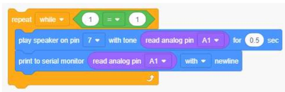
This tells the Arduino to play the speaker connected to pin 7 with a sound that's controlled by the value the photoresistor is sending to pin A1. You can then test your code by clicking "Start Simulation" on Tinkercad.
